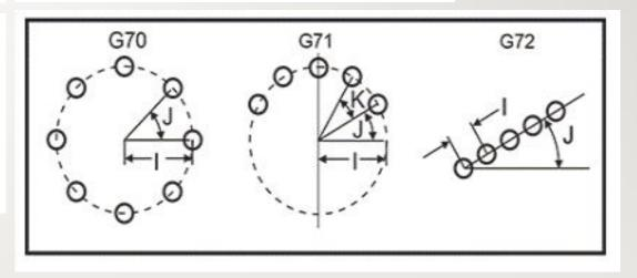
\*These are non-modal G codes that must be used with one of the canned cycles G73, G74, G76, G77, or G81-G89. A canned cycle must be active so that at each position, a drill or tap function is performed. See also G-code Canned Cycles section.
